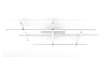
Ceiling lighting fixture for interiors, with direct and indirect light emission. Pickled sheet metal ceiling bracket in polyacrylic paint. Pickled sheet metal wall plate in polyacrylic paint. Extruded aluminium structure in white, mat black, bronze, mat brass or titanium polyacrylic paint. Joints in turned brass and die-cast aluminium in polyacrylic paint. Die-cast aluminium end caps in polyacrylic paint. Extruded polycarbonate diffusers with opaline finish.
