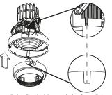
install the filterholder again by first alining A and B
