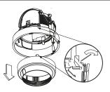
Bend the springs to remove the filterholder.
