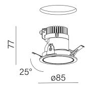
Tolerance for dimensions ± 1mm
