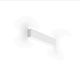
Wall lighting fixture for interiors, with direct and indirect light emission. Extruded aluminium structure in RAL 9003 white or black powder paint. Extruded polycarbonate diffusers with opaline finish. Pickled sheet metal end caps in polyacrylic paint.
